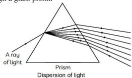
When do the light rays get refracted? (I) As the light ray enters the prism from the air.
