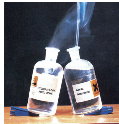
Figure 30. Ammonia combines with hydrochloric acid to form dense white fumes of ammonium chloride.
