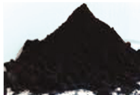
Figure 19. This is iron (II, III) oxide. When heated iron metal reacts with steam, it forms iron (II, III) oxide.
