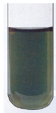
(b) When sulphur dioxide gas is passed through potassium dichromate solution, the orange colour of potassium dichromate solution changes to green.
