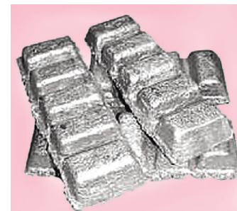
Figure 54. Zinc metal formed by the reduction of zinc oxide with carbon (or coke).
