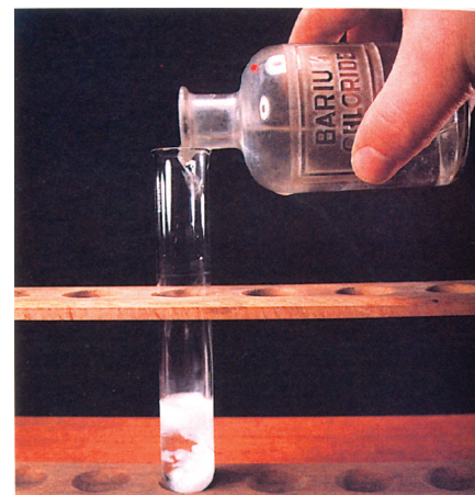
Figure 48. On mixing barium chloride solution with sodium sulphate solution, a white precipitate of barium sulphate is formed along with sodium chloride solution.
