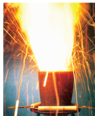
Figure 46. The displacement reaction between iron (III) oxide and powdered aluminium produces so much heat that iron metal obtained is in molten form.
