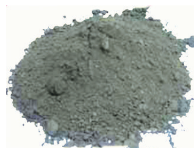
Figure 16. This is manganese dioxide ( \text{MnO}_2 ). It is used as a catalyst during the preparation of oxygen gas from potassium chlorate.
