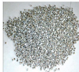
Figure 13. This picture shows zinc metal in the form of zinc granules. Zinc metal is a solid, so we write Zn (s) for it in a chemical equation.
