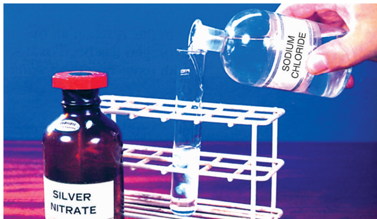
Figure 47. On mixing sodium chloride solution with silver nitrate solution, a white precipitate of silver chloride is obtained along with sodium nitrate solution.
