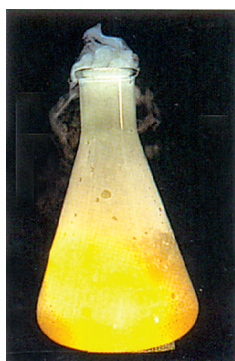
Figure 25. Sodium burns in chlorine to form sodium chloride.
