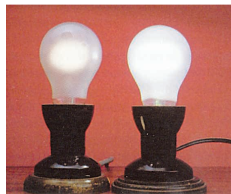
Figure 33. The bulb on left side has higher resistance, so its power is less. It glows less brightly. The bulb on right side has less resistance, so its power is more. It glows much more brightly.
