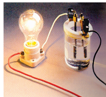
Figure 21. A strong acid (say, hydrochloric acid) has a high electrical conductivity, so the bulb glows brightly.
