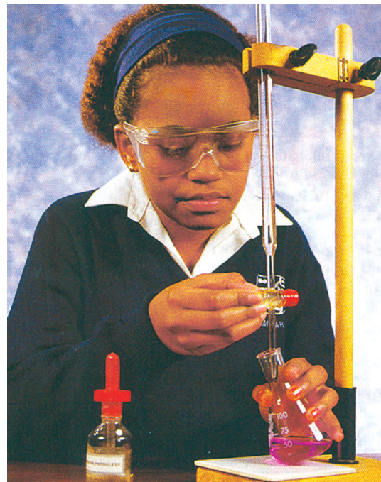
Figure 15. This student is carrying out the neutralisation reaction between sodium hydroxide solution and hydrochloric acid solution. She has taken sodium hydroxide solution (containing phenolphthalein indicator) in the conical flask and adding hydrochloric acid to it from the burette. The acid will be added to sodium hydroxide solution until the indicator just changes colour : from pink to colourless.
