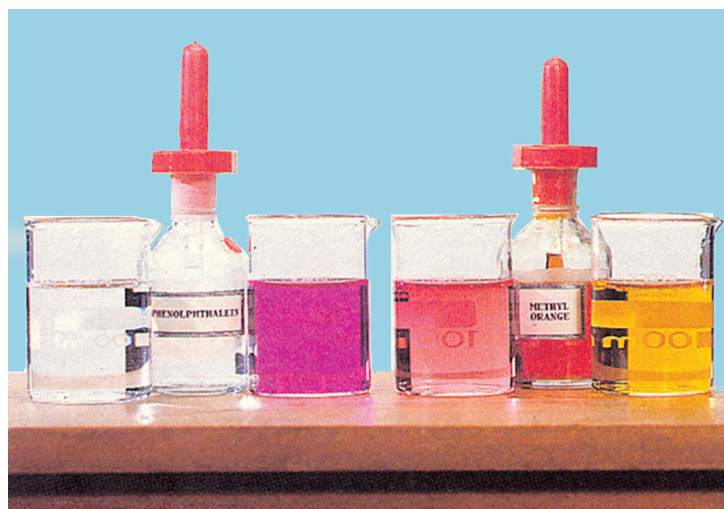
Figure 3. The bottle (with dropper) on the left side in this picture contains phenolphthalein indicator. Phenolphthalein indicator is colourless in acid solution but turns pink in basic solution. The bottle on the right side in the above picture contains methyl orange indicator. Methyl orange indicator is red in acid solution but yellow in basic solution.
