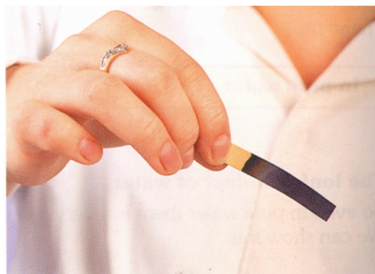
Figure 30. A solution has turned this universal indicator paper violet showing that it is a strong base (or strong alkali).
