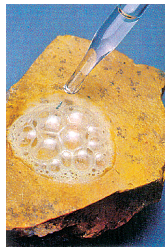
Figure 14. Limestone is calcium carbonate. Carbon dioxide is formed when an acid is dropped onto the surface of limestone. This reaction is a convenient test for limestone.
