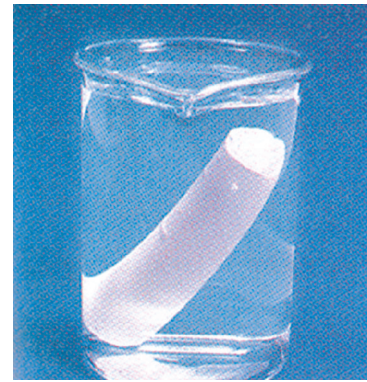
Figure 35. White phosphorus is stored under water because it burns spontaneously in air but does not react with water.
