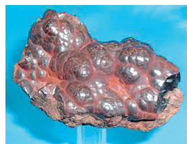
Figure 72. This is an iron ore called haematite. It contains iron (III) oxide, \text{Fe}_2\text{O}_3 .
