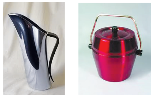
Figure 89. These pictures show two objects made of anodised aluminium to prevent their corrosion.
