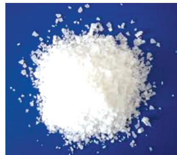
Figure 53. Magnesium chloride ( \text{MgCl}_2 ) is an ionic compound containing ionic bonds which is made up of magnesium ions ( \text{Mg}^{2+} ) and chloride ions ( \text{Cl}^- ) held together by electrostatic force of attraction.
