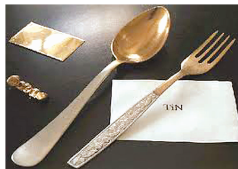
Figure 47. Because of its metallic gold colour, titanium nitride (TiN) is used for giving decorative coatings to iron and steel objects.
