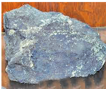
Figure 81. This is the copper ore called copper glance. It contains copper (I) sulphide, \text{Cu}_2\text{S} .
