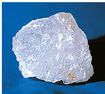
Figure 74. This is a sodium ore called 'rock salt'. It contains sodium in the form of sodium chloride, NaCl.
