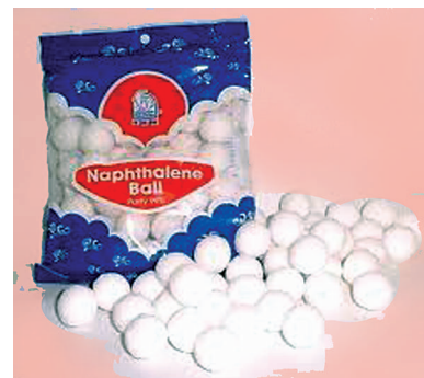
Figure 70. These are naphthalene balls. Naphthalene is a covalent compound. It has a low melting point of 80^{\circ}\text{C} . Naphthalene is also insoluble in water.
