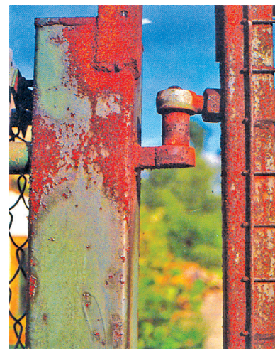
Figure 85. The corrosion of iron is called rusting. Rusting eats up iron objects gradually and makes them useless. This picture shows a rusted iron gate post.
