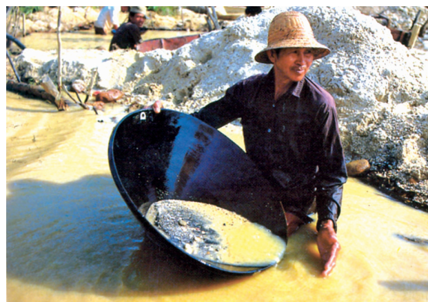
Figure 71. Some metals such as gold are very unreactive due to which they can be found in their metallic form in the Earth's crust. On a small scale, gold is extracted by panning (which involves washing the gold containing gravel in a pan to separate out gold).
