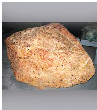
(a) This is aluminium ore called bauxite. It contains hydrated aluminium oxide, \text{Al}_2\text{O}_3 \cdot 2\text{H}_2\text{O}
