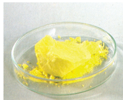
Figure 32. This is sulphur. Sulphur burns in air to form an acidic gas sulphur dioxide.
