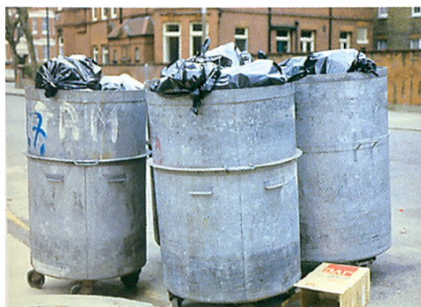
(a) These bins made of steel have been galvanised (coated with zinc metal)
