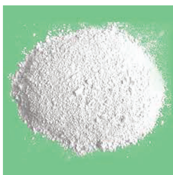
(b) This is purified aluminium oxide (which has been obtained from bauxite ore)
