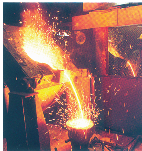
Figure 93. To make an alloy, the molten metals are mixed, then allowed to cool.
