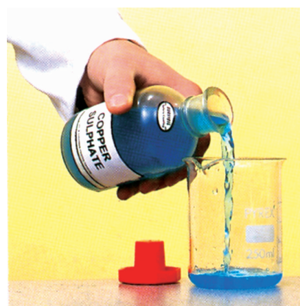
Figure 67. Copper sulphate is a blue coloured ionic compound. So, it dissolves in water to form a blue coloured copper sulphate solution.
