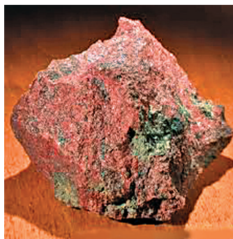
Figure 79. This is a mercury ore called cinnabar. It contains mercury (II) sulphide, \text{HgS} . Mercury metal can be obtained by simply heating this cinnabar ore in air.
