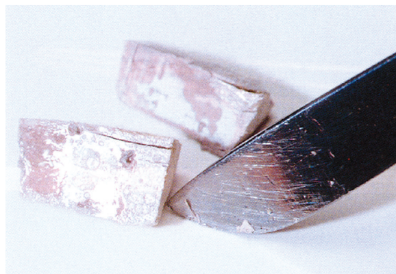
Figure 10. Sodium metal is so soft that it can be easily cut with a knife.
