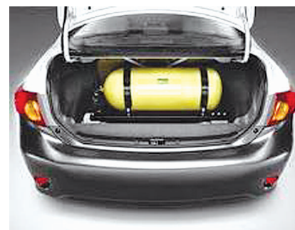
Figure 38. Natural gas is an excellent fuel which does not cause much air pollution. Many cars, buses and autos in Delhi run on compressed natural gas (CNG). This picture shows a CNG cylinder fitted in the boot of a car.
