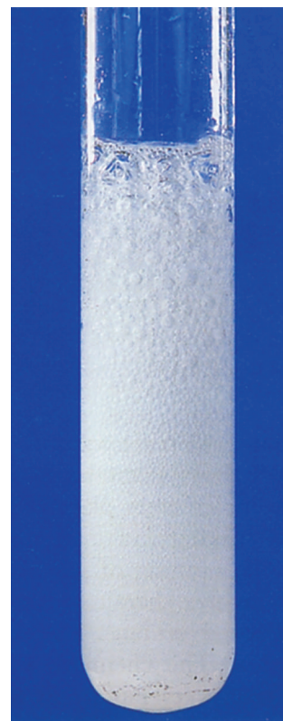
Figure 52. Ethanoic acid reacts with sodium hydrogencarbonate to produce brisk effervescence of carbon dioxide gas.
