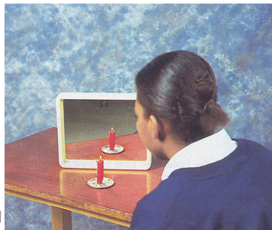
Figure 15. The image of candle in the plane mirror is the same distance behind the mirror as the candle is in front of the mirror.
