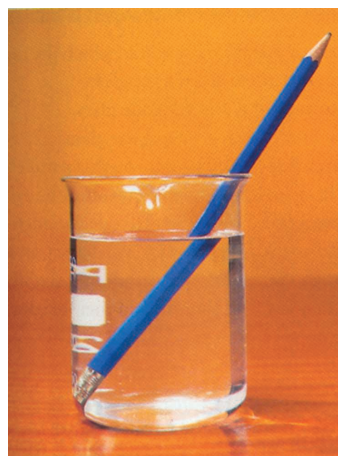
Figure 12. The pencil is partly immersed in water. Because of the refraction of light coming from the part of the pencil that is under water, the pencil appears bent.
