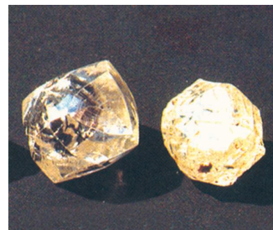
Figure 18. Diamonds sparkle partly because of their high refractive index. The shape to which they are cut also helps them to sparkle.
