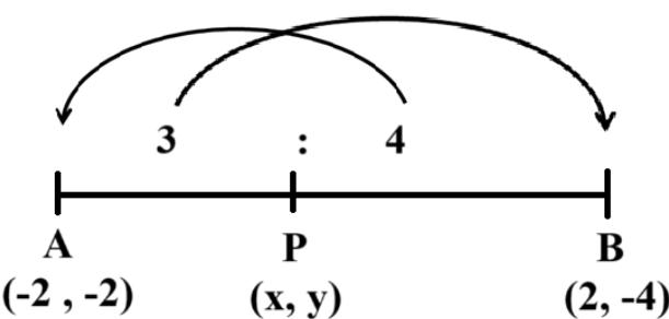
$P(x, y)$ divides AB in the ratio 3:4<br>$x = \frac{3 \times 2 + 4 \times (-2)}{4+3} \Rightarrow x = -\frac{2}{7}$                                                                                                                                                     | $\frac{1}{2}$<br>$\frac{1}{2}$                                   |
